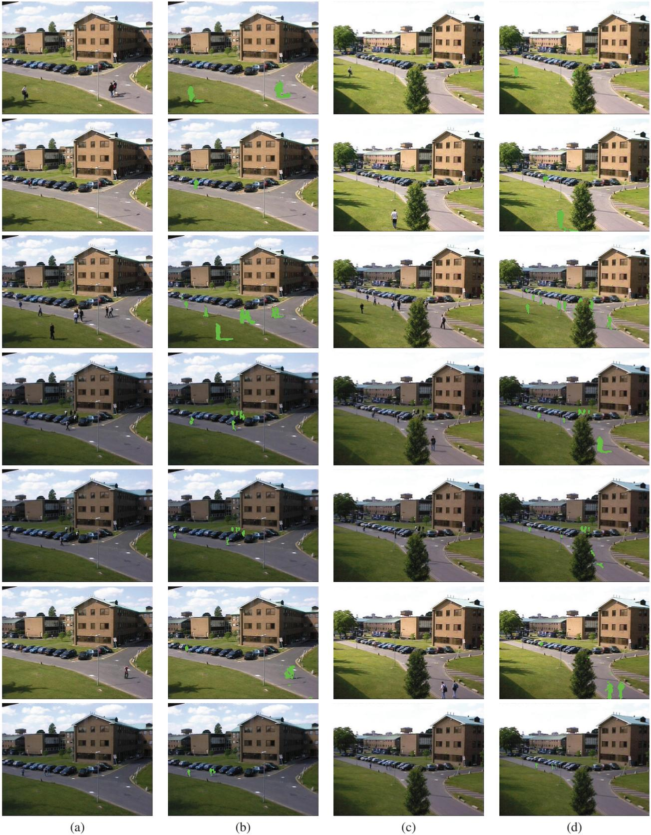
Fig. 1. Selected frames from sequence *Dataset3*: (a) Original frame from Camera1 and (b) corresponding moving object detection result achieved by the 3D\_SOBS algorithm (green pixels); (c) Original frame from Camera2 and (d) corresponding moving object detection result achieved by the 3D\_SOBS algorithm.
